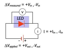
e) In the "Current vs. Voltage" panel, sweep the voltage from 0-3 Volts, in 100 or 200 steps. You should see a curve like that on the first page. Do this for both LEDs.
