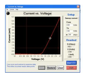
When measuring I versus V, as above, the LED will show almost no current until a specific "threshold" voltage is reached, after which the current increases rapidly and the LED begins to glow. Roughly, what should this threshold voltage be?
