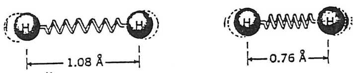
Figure 12 Molecular vibrations—a measure of bond order. (a) Greatly expanded view of the bottom of the energy curves of Figure 10 showing the energy required for a 0.1 \text{ \AA} change in bond length. (b) Ball-and-spring model shows a weak spring in H_2^+ and a stiff spring in H_2 .
