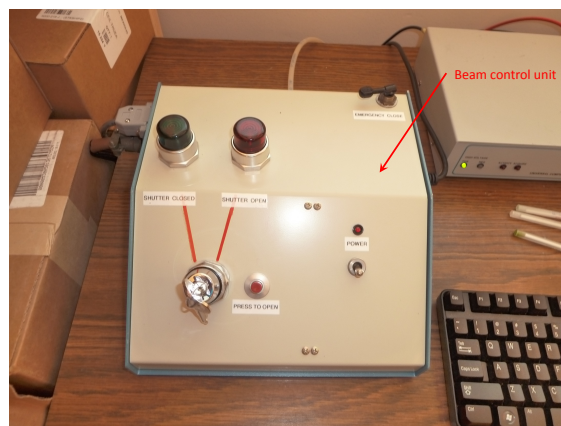
Figure 10.4: Beam control unit used to release the \gamma -ray beam.
