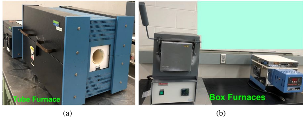
Figure 2.2: (a) Tube, and (b) box furnaces used for thermal treatments of the Heusler samples.
