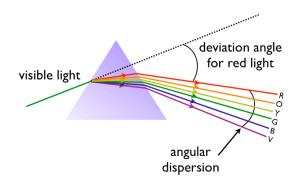
**Solution:** What we need to do is find the deviation angle for both red and violet light in terms of the incident angle and refractive index of the prism. The angular dispersion is just the difference between the deviation angles for the two colors. First, let us define some of the geometry a bit better, referring to the figure below.
