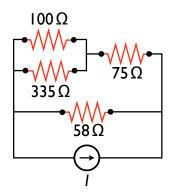
25. What is the equivalent resistance of the arrangement of resistors at left? You do not need to include the current source in your analysis
