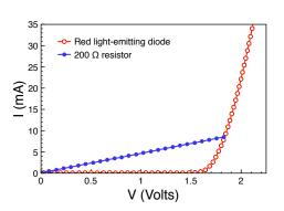
26. The figure at right shows the current-voltage relationship for a light-emitting diode (LED) and a resistor. When the voltage is 1.7 V, which has the **higher resistance**? *Hint: what does the slope of this plot mean*?
