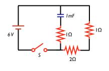
20. The switch S is suddenly closed in the circuit at left. The capacitor is uncharged before the switch is closed. After a very long time, what will be the steady-state current in the  $2\Omega$  resistor? *Hint: what is the capacitor doing after a long time?*
