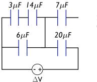
12. What is the equivalent capacitance for the five capacitors at left (approximately)?
