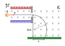
13. Consider the mass spectrometer shown at left. The electric field between the plates of the velocity selector is  $|\vec{\mathbf{E}}| = 1000 \text{ V/m}$ . What must the magnitude of the magnitude of the magnetic field be, if r = 4.6 cm for a it singly-charged ion with  $m = 7.3 \times 10^{-26} \text{ kg}$ ?
