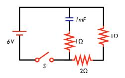
22. The switch S is suddenly closed in the figure at left. After a long time compared to the time constant of the capacitor, what will the current be in the  $2\Omega$  resistor? Hint: what is the capacitor doing after a long time?
