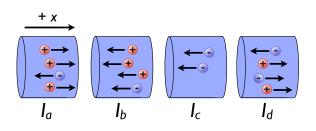
13. Consider the positive and negative charges moving horizontally through the four regions at left. Rank the magnitudes of the currents in these four regions from highest to lowest. Positive current is defined as positive charges moving in the +x direction.
