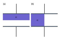
4. A parallel plate capacitor has a capacitance C when there is vacuum between the plates. The gap between the plates is half filled with a dielectric with dielectric constant  $\kappa$  in two different ways, as shown below. Calculate the effective capacitance, in terms of C and  $\kappa$ , for both situations. Hint: try breaking each situation up into two equivalent capacitors.
