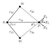
Rather than worry about which nucleus is which, we will simply label the charges  $q_1$ ,  $q_2$ , and  $q_3$  and be as general as possible. We will also label the distances in a generic but self-explanatory way: the distance from charge 1 to charge 2 is  $r_{12}$ , the distance from charge 3 to the point P is  $r_{3p}$ , and so on.
