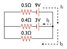
In this case, there are three currents to deal with, it is the third  $I_3$  that we are interested in. First, we can apply the "junction rule" at the circular dot on the right-hand side of the circuit. Current  $I_1$  enters the junction, currents  $I_2$  and  $I_3$  leave:
