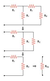
Now we only have  $R_3$  and one  $R_1$  left, purely in series. Combining them will give us one single equivalent resistor  $R_{eq}$ :
