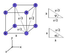
By symmetry, the x, y, and z components of the electric force must be equal. Thus, we only need to calculate one component of the total force on the charge of interest. We will choose the coordinate system as indicated in the figure, and calculate the x component of the force on the lower right-most charge. We can already see that several charges will not give an x component of the force at all, just from symmetry - charges 3, 4 and 7. This leaves only charges 1, 2, 5, and 6 to deal with.
