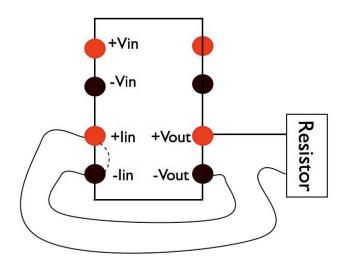
One end of the resistor goes to "+Vout, the other goes to "+lin". Then "-lin" connects back to "-Vout." Why are the connections this way?
