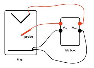
**Connect the electrodes** to  $+V_{out}$  and  $-V_{out}$  on your lab box. Make the flat electrode negative (connected to  $-V_{out}$ , black terminal). This will supply the potential difference between your two electrodes.
