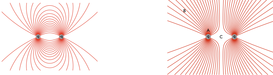
Figure 3.6: left Field lines for two equal and opposite charges, an “electric dipole.” The number of lines leaving the positive charge equals the number terminating at the negative charge right Field lines for two positive charges of equal magnitude. Can you rank the relative field strengths at points A, B, and C? xi
