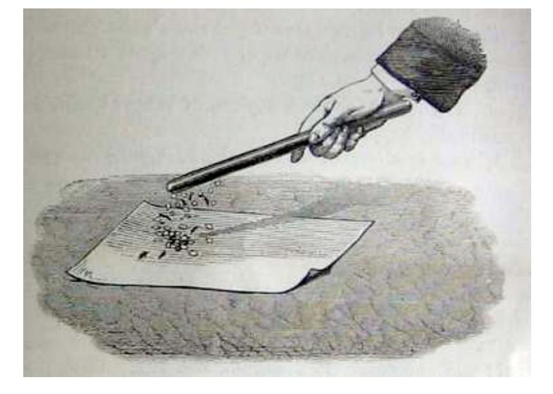
"Little pieces of tissue paper (or light grains of sawdust) are attracted by a glass rod rubbed with a silk handkerchief (or by a piece of sealing wax or a rubber comb rubbed with flannel)."
