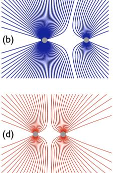
**9.** Which set of electric field lines could represent the electric field near two charges of the same sign, but different magnitudes?
