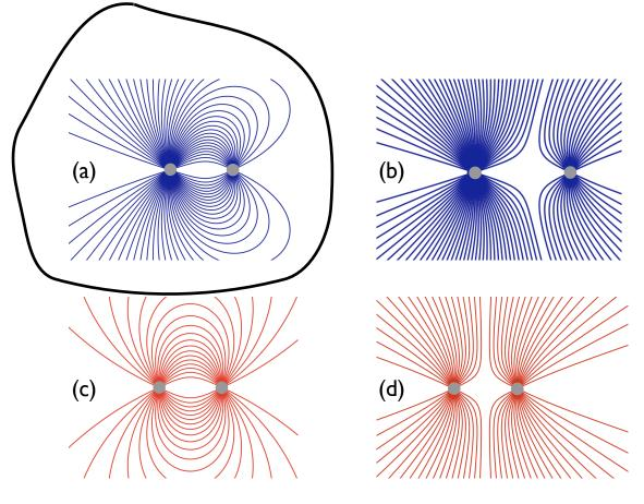
**10.** Referring again to the figure above, which set of electric field lines could represent the electric field near two charges of *opposite sign* and *different magnitudes*?
