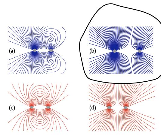
**9.** Which set of electric field lines could represent the electric field near two charges of the same sign, but different magnitudes?
