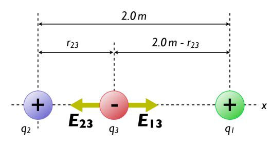
2. Three point charges lie along the x axis, as shown at left. A positive charge  $q_1 = 15 \,\mu\text{C}$  is at  $x = 2 \,\text{m}$ , and a positive charge of  $q_2 = 6 \,\mu\text{C}$ is at the origin. Where must a *negative* charge  $q_3$  be placed on the x-axis **between the two positive charges** such that the resulting electric force on it is zero?
