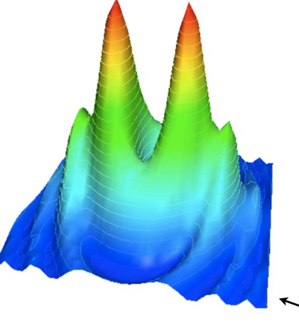
x, y = spatial coordinates z = electric potential 3d equipotential lines? contours of constant V
