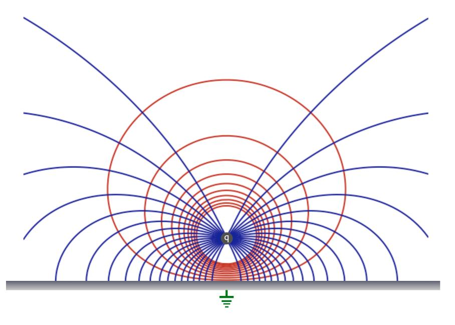
conductor = mirror for field & potential lines
