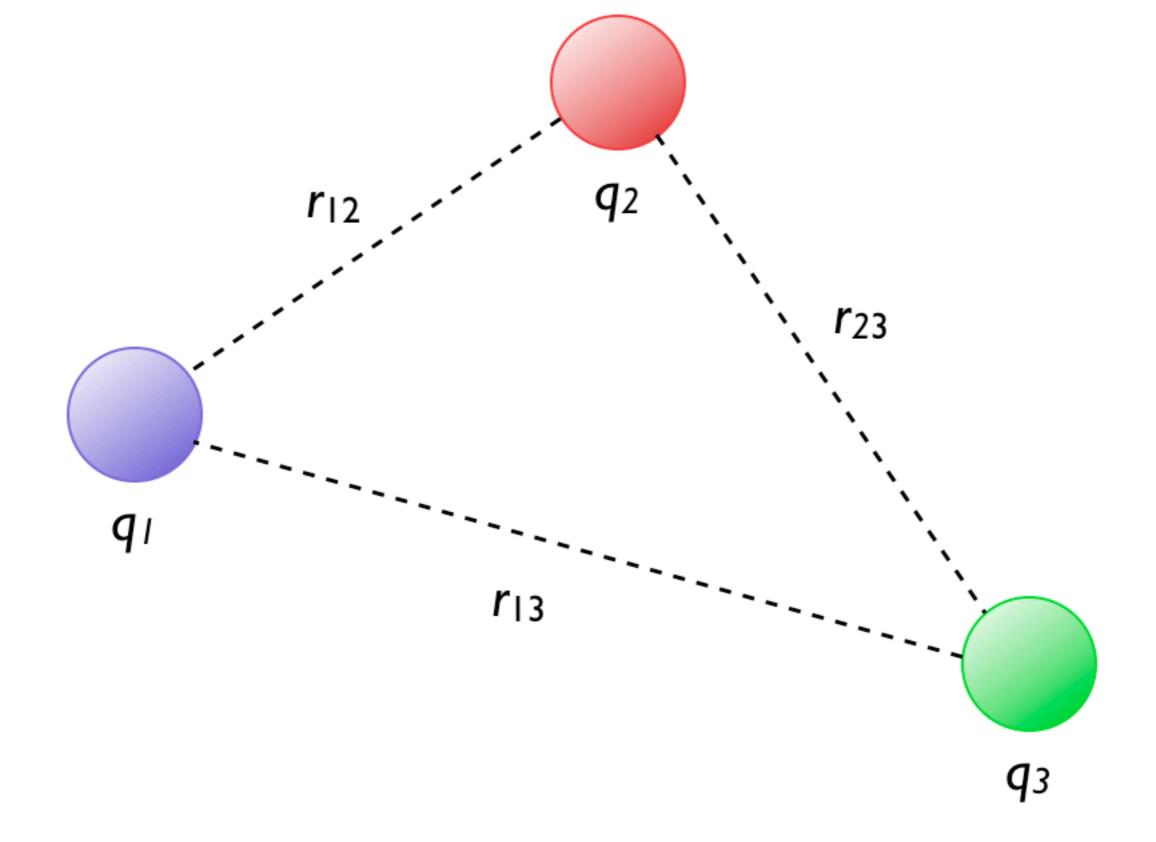
$$PE = PE_{1\&2} + PE_{2\&3} + PE_{1\&3} = PE_{2\&1} + PE_{3\&2} + PE_{3\&1} = k_e \left(\frac{q_1q_2}{r_{12}} + \frac{q_1q_3}{r_{13}} + \frac{q_2q_3}{r_{23}}\right)$$
