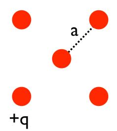
$PE_{\text{square}} = 4 \text{ (energy of center-corner pair)} + 2 \text{ (energy of far corner pair)} + 4 \text{ (energy of adjacent corner pair)}$
