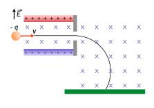
**3.** The figure shows a simplified mass spectrometer. Particles with charge q and mass m enter at left with a velocity v, and encounter a region with both an E and B field as shown. What is the relationship between v, B, and E for particles that make it through the aperture in the middle of the detector?
