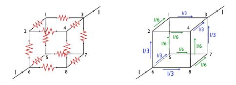
Take any corner, and let a current I enters at that node. It then has a choice of three directions to go along the cube edges. Each path has an identical resistance, so the current must split up evenly with I/3 through each. Likewise, the current exiting the node on the opposite corner comes from three resistors, each with a current I/3. This leaves 6 resistors in the middle that must share the whole current I. Because each of those is also identical, they must each have current I/6.
