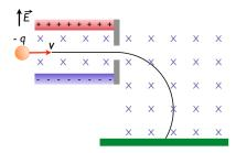
3. The figure shows a simplified mass spectrometer. Particles with charge q and mass m enter at left with a velocity v, and encounter a region with both an E and B field as shown. What is the relationship between v, B, and E for particles that make it through the aperture in the middle of the detector?
