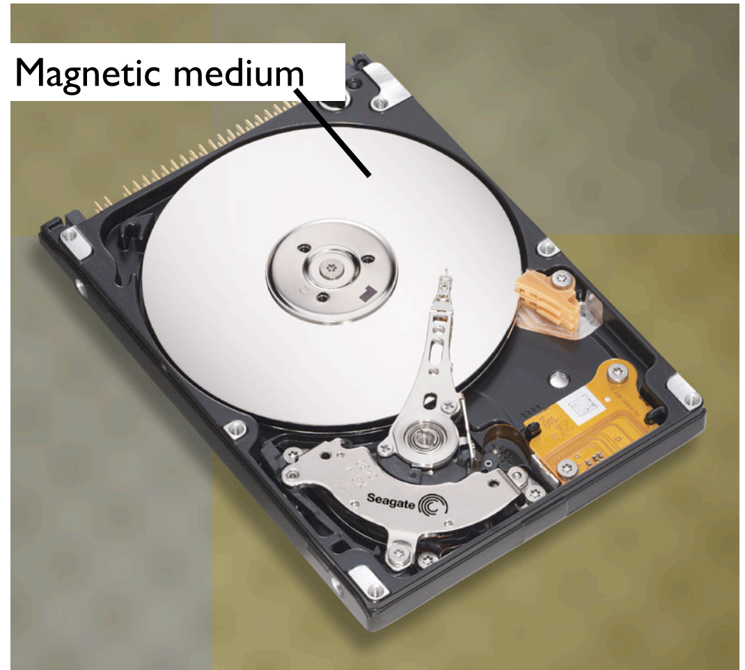
160 Gbit 2.5" perpendicular drive for laptops
