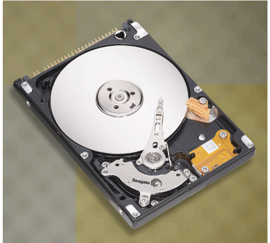
160 Gbit 2.5" perpendicular drive for laptops
