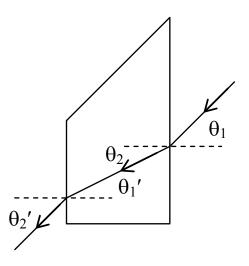
**Now trace the lines**. Place a piece of white paper under the apparatus, and use a pencil to indicate points on the path of the ray. For instance, make a dot where the ray leaves the light source, where it hits the plastic, where it leaves the plastic, and where it is about an inch away from the plastic. You'll also need to trace the right surface of the trapezoid. Then connect the dots to show the lines followed by the light ray.
