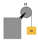
**Solution:** In order to get acceleration and angular acceleration, we'll need to use force and torque, respectively. Start with the pulley. The tension T in the rope pulls on the edge of the disk a distance R from the center of rotation at an angle of  $\theta_{RT} = 90^{\circ}$ , which causes a torque  $\tau$ . This torque must equal the disk's moment of inertia times the angular acceleration.
