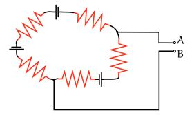
2. In the circuit above, all five resistors have the same value,  $100 \Omega$ , and each battery has a rated voltage of 1.5 V and no internal resistance. Find the open-circuit voltage and the short-circuit current for the terminals A, B. Then find the Thèvenin equivalent circuit (i.e., the ideal battery and resistor that could replace this circuit between terminals A, B.)
