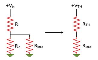
**Solution:** With no load attached, the output voltage is just the voltage across  $R_2$ . Since we have only two series resistors, the current in both is the same, and it must be  $V_{in}/(R_1+R_2)$ . The output voltage is then
