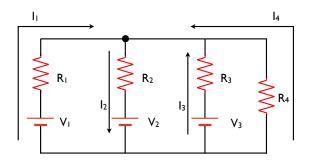
Now we just apply conservation of charge (current) and energy (voltage). We have 4 loops which will give us three conservation of energy equations, and 4 unknown currents. That means we need a single node equation based on conservation of current, which we can apply at the point indicated by the dot in the figure above:
