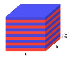
$\rho = 1/\sigma$ . We will also say the tin layers have thickness  $t_1$ , and the silver layers thickness  $t_2$ . The total thickness of our entire multi-layer stack is then  $t_{tot} = n_1 t_1 + n_2 t_2$ .
