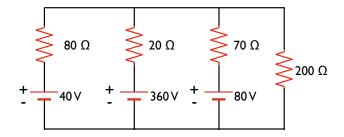
**Solution:** First we must label the currents in each branch and pick their directions. We will pick the directions arbitrarily - in fact, we will intentionally choose directions that are extremely unlikely to be correct just to drive home the point that it doesn't matter at all. If we chose the current direction in a particular branch incorrectly, the current comes out negative, so it really doesn't
