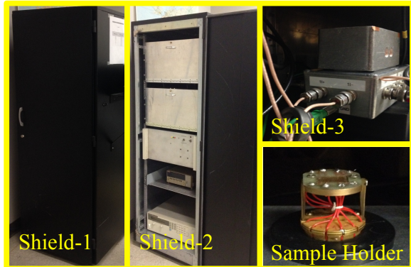
FIG. 12. Shielding the instrument and the device under the test from environmental electromagnetic interference. Two layers of shielding, shield 1 and 2 contain the all components of the analyzer, and the third layer of shielding around the sample holder further minimizes external influences.
