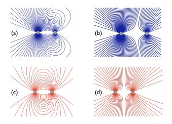
Set (b). If the charges are of the *opposite* sign, then the field lines would have to run from one charge directly to the other. Field lines start on a positive charge and end on a negative one, and there should be many lines which run from one charge to the other. Since opposite charges attract, the field between them is extremely strong, the lines should be densest right between the charges. This is the case in (a) and (c), so they are not the right ones.
