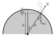
Once the boy is at a given angle  $\theta$ , his height above the ground will be  $h = R \cos \theta$ , meaning he has moved downward from his starting position by an amount  $\Delta h = R - h$ . The boy's weight mg will be acting downward making the same angle  $\theta$  with respect to a radial line at that point, while the normal force N will act in the positive radial direction.
