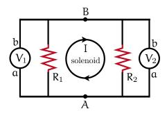
$\square$  5. Given the circuit below, show that if the condition  $R_1R_2 = L/C$  is satisfied, the difference in voltage between points A and B will be zero at *any* frequency.
